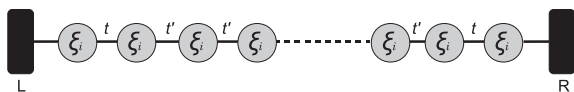
Fig. 2. Effective one-dimensional model: linear monoatomic chain of N sites connected to two metallic leads.
